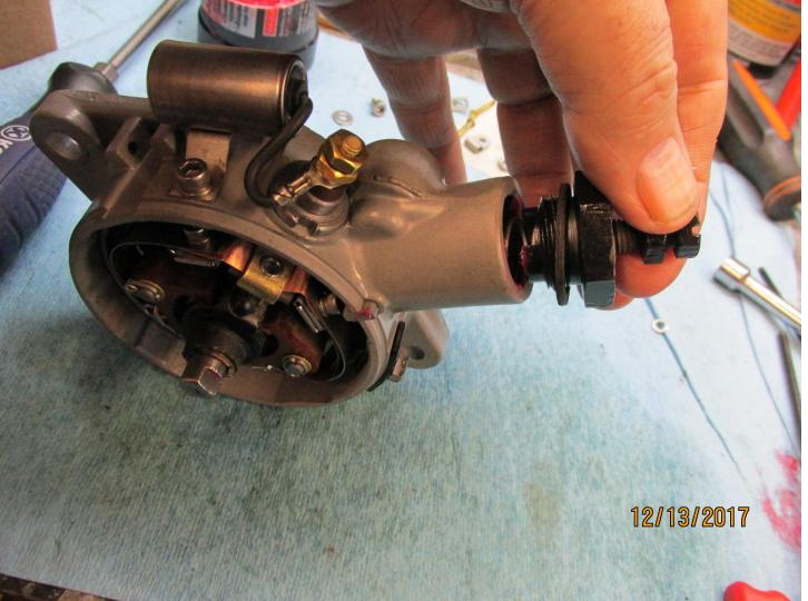
The last item to be adjusted and installed is the Vacuum brake.
