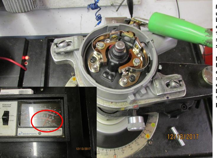
Passenger side is then unlocked and total of both sets (dwell) is adjusted to 36 degrees to provide proper coil saturation for good spark.
