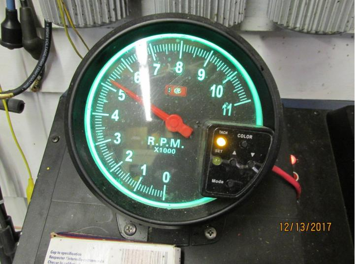
We then run the unit at 5000 rpm for a period of time. After testing thousands of these you know when they are right and wrong based on the hum or noise the unit makes .
