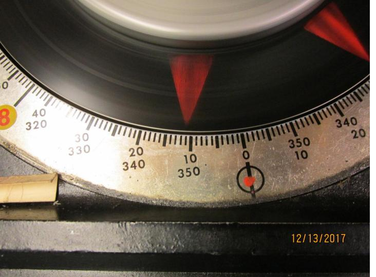
The crab unit is a 11 degree distributor . 11 degrees at approx 2000 rpm = 22 degrees of engine timing.
