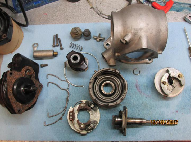
Tear down of early 3 bolt housing with 3 bolt coil.
