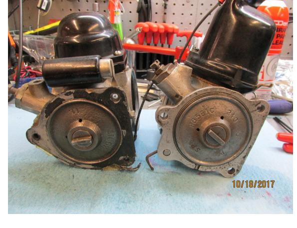
Basically there are two housings and designs for the model years 32-thru 1941. The 32 is somewhat different and will be covered as a seperate unit along with the oblong coil for the 1936 model year. However for the most part we will cover the two units shown.... I call them the 3 bolt with 3 bolt coil and a 4 bolt with 2 bolt coil.
