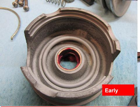
Early rear housing shown (left upper) and later smooth unit shown. Upper unit shows ribs to be used with oil deflector and early drive shaft. Both of these are very good and very seldom need bushing replacement. Bushings are available if needed.
