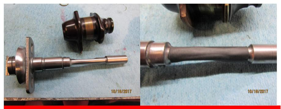
Rotor shaft is cleaned, polished and center (under rotor) is insulated with shrink tubing. Spark will always take the path of least resi8stance and will try at times to go to center shaft. For the most part these rotors work very well and last a long time. I usually clean and inspect, looking for any sign of burning or arcing. Clean, polish brass ends and use them...... Some aftermarket replacements are very poor quality!!
