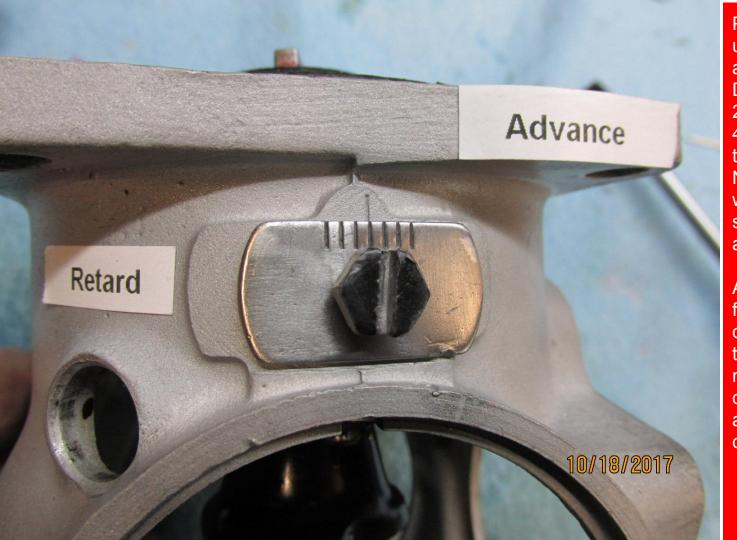
Properly set up is usually one mark advanced to provide 4 Degrees BTDC.
