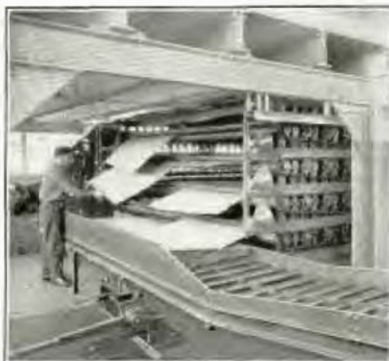
Paper Comes in Large Wet Sheets. Drying is Done in Long Ovens.
