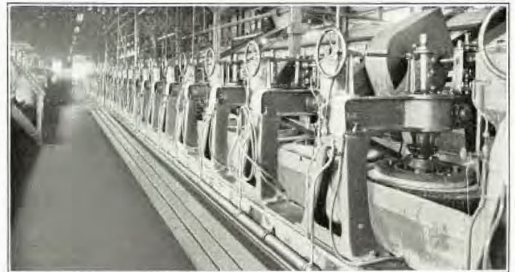
Glass Grinding Machines Made of Standard Ford Parts. Note the Ford Steering Wheels and Gears.
