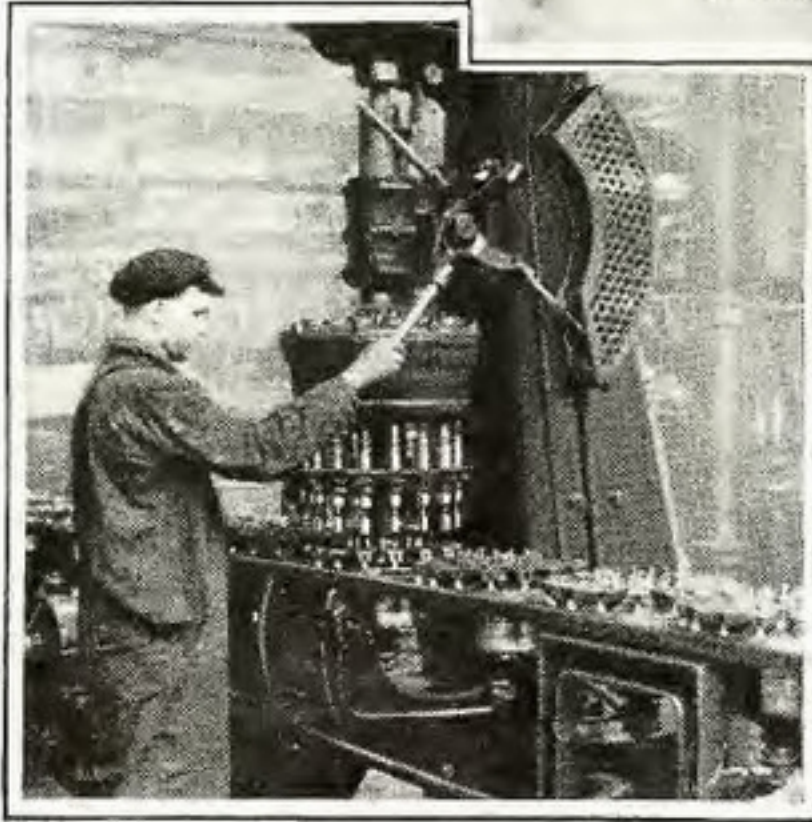
Setting all the Magneto Screws at once
