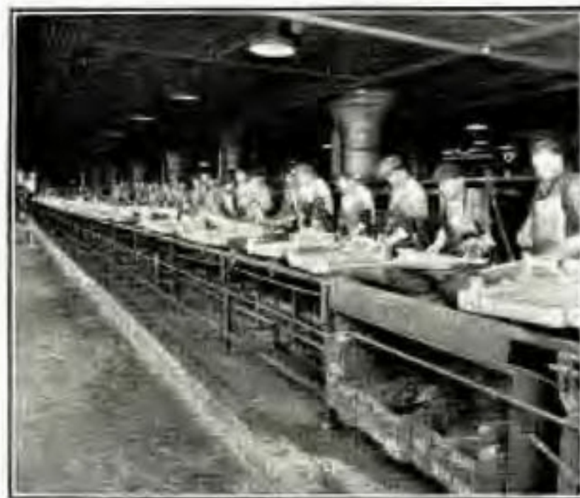
Each Radiator Tested For Leaks
