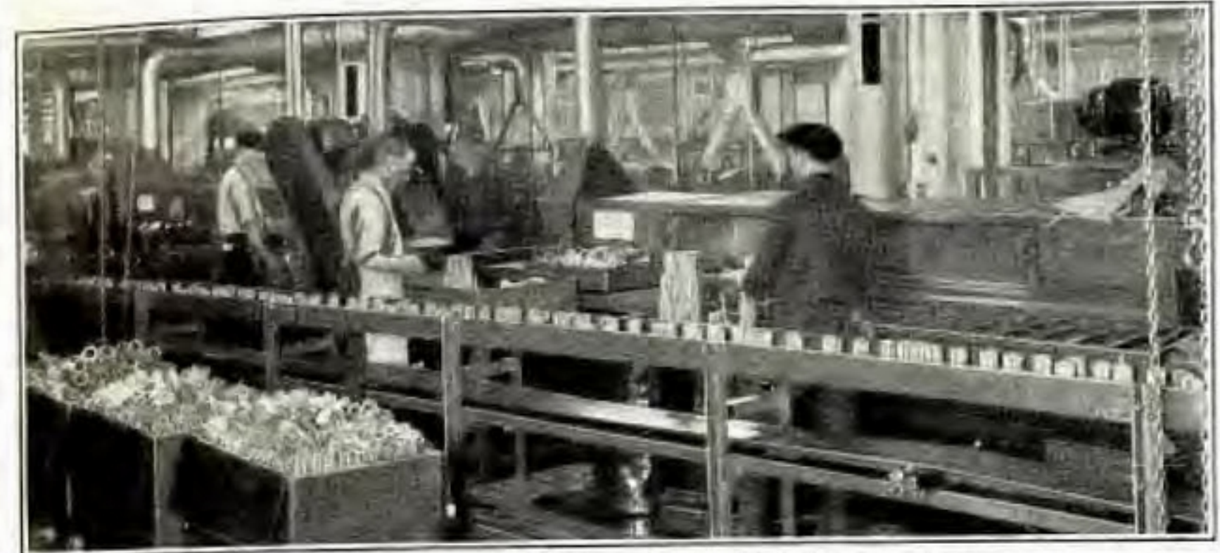
Bearings Conveyed Away After Final Inspection
