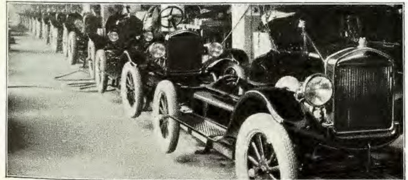
Ford Final Assembly Conveyors are Standardized the World Over
