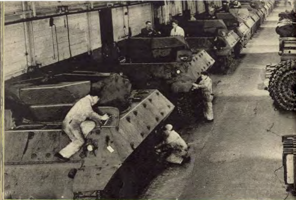
This is a telescopic view of the tank assembly lines at Highland Park. On the left are the M-10 Tank Destroyers and on the right M-4 General Shermans near completion.
