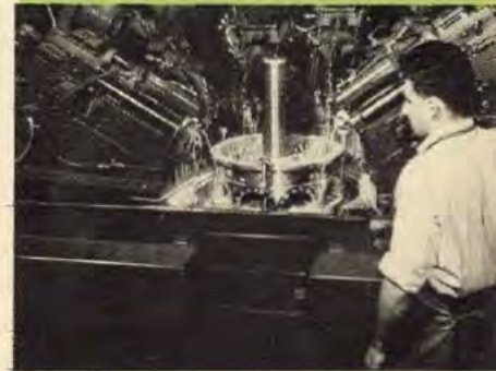
This electronically-controlled tool prevents breakage as it drills small holes.
