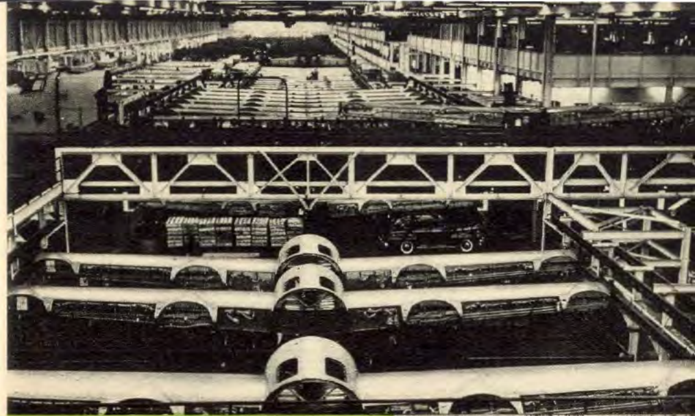
An automobile is dwarfed by the center wing section. This view gives an impression of Ford automotive assembly methods adapted to mass production of aircraft.
