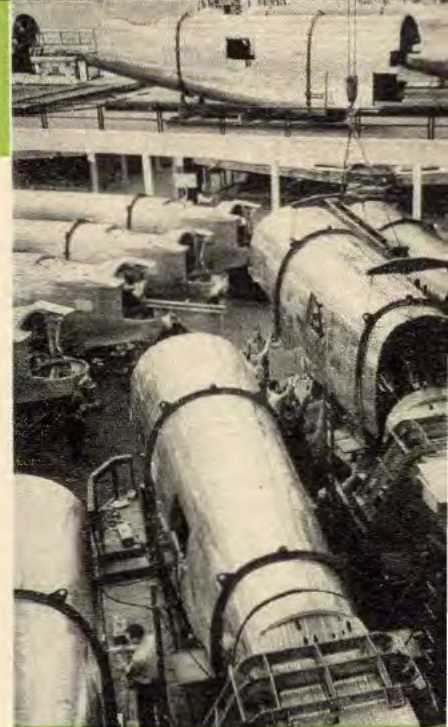
Fuselage sections gleam under fluorescent lights ready to move to final assembly. Extra sections are on balcony.
