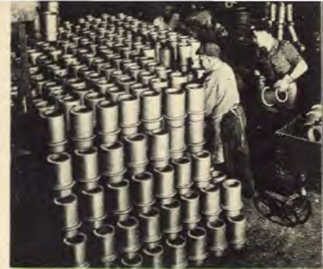
Centrifugal casting of cylinder barrels results in better quality, less machining, and saves metal. It is a Ford innovation.
