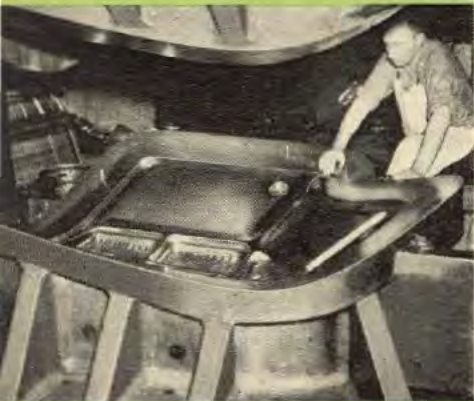
Use of hard steel dies, shown in the press, increased Willow Run capacity.
