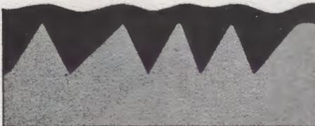
Figure 57—If sanded level before all solvents have evaporated further evaporation of solvents will cause a shrinkage leaving furrows over sand marks in metal.
