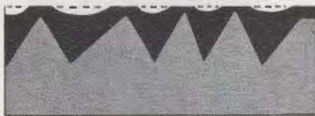
Figure 56—Primer surfacer applied over sanded metal simulates the contours of the metal, shrinkage being more over deeper fills.
