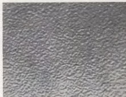
Figure 106—Orange Peel
