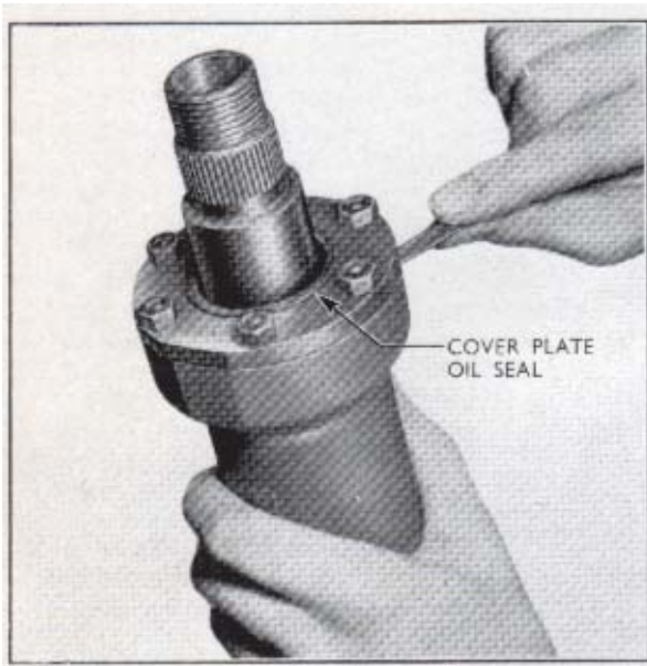
Fig. 11 Steering Main Nut Bearing Adjustment
