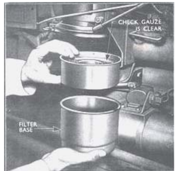
Fig. 4 Removing the Air Cleaner Base
