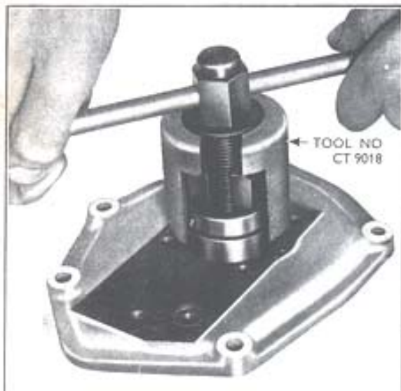
Fig. 14 Removing the Camshaft Outer Races
