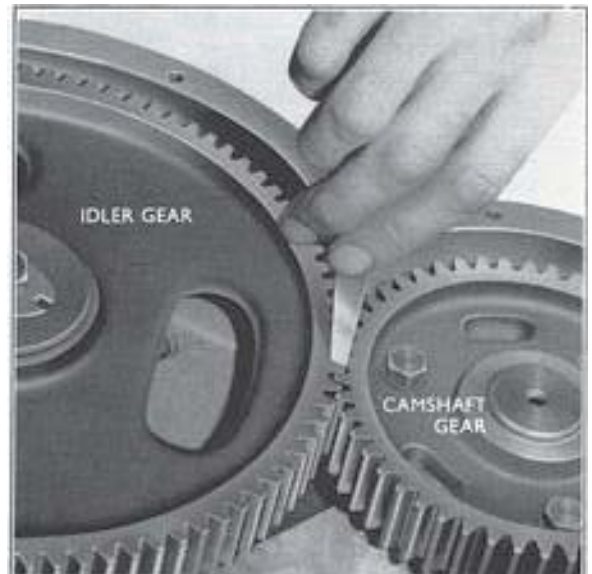
Fig. 9 Checking Timing Gear Backlash
