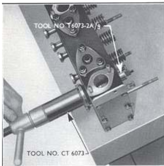
Fig. 6 Replacing a Valve Guide
