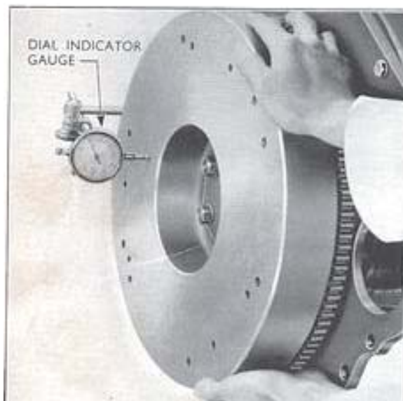
Fig. 18 Checking Flywheel "Run-Out"
