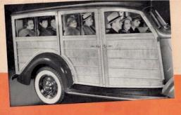
Front and rear seats each accommodate three. The center seat is double width, leaving ready access to rear. Rear seat can replace center seat, providing room for six with unusually large luggage space, or both center and rear seats can be removed completely.
