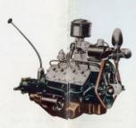
This is the Ford V · · · 8 60-horsepower engine—the most economical Ford engine ever built. Except in size and power it is the same basic design as the Ford V · · 8 85-horse ower engine, used and approved by more than four million motorists. The Ford V · · 8 engine brings fine-car performance to the low-price, low-cost field—within the means of all who can afford any new car. The brilliant "85" gives top performance; the thrifty "60" rock-bottom gasoline economy.
