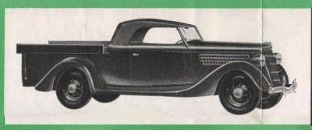
FORD V-8 ROADSTER WELL-TYPE UTILITY MODEL 304—Body has extensive loading space. Designed for the use of station-owners, contractors, engineers, etc. Of handsome appearance this unit has a wide range of usefulness in town or country service. Auxiliary rear springs optional equipment. Loading dimensions:—Length. 77 inches. Width at floor, 56 inches. Height, including sideboards, 22½ inches.
