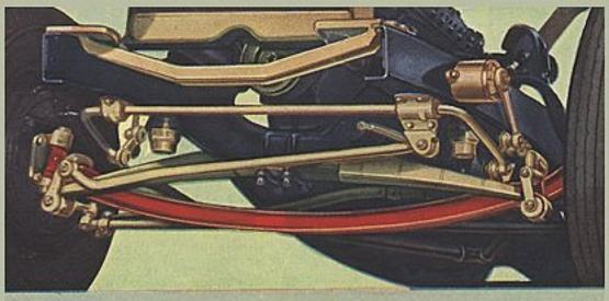
Mercury's double-action hydraulic shock absorbers are of improved design—slow-motion springs are longer than ever—for increased riding comfort. Mercury's new transverse stabilizer and anti-sway bar improve car equilibrium—minimize side-sway—provide better steering control.
