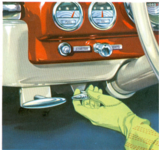
Convenient knob on instrument panel permits overdrive to be locked "in" or "out". When knob is "in", overdrive is in operation.
