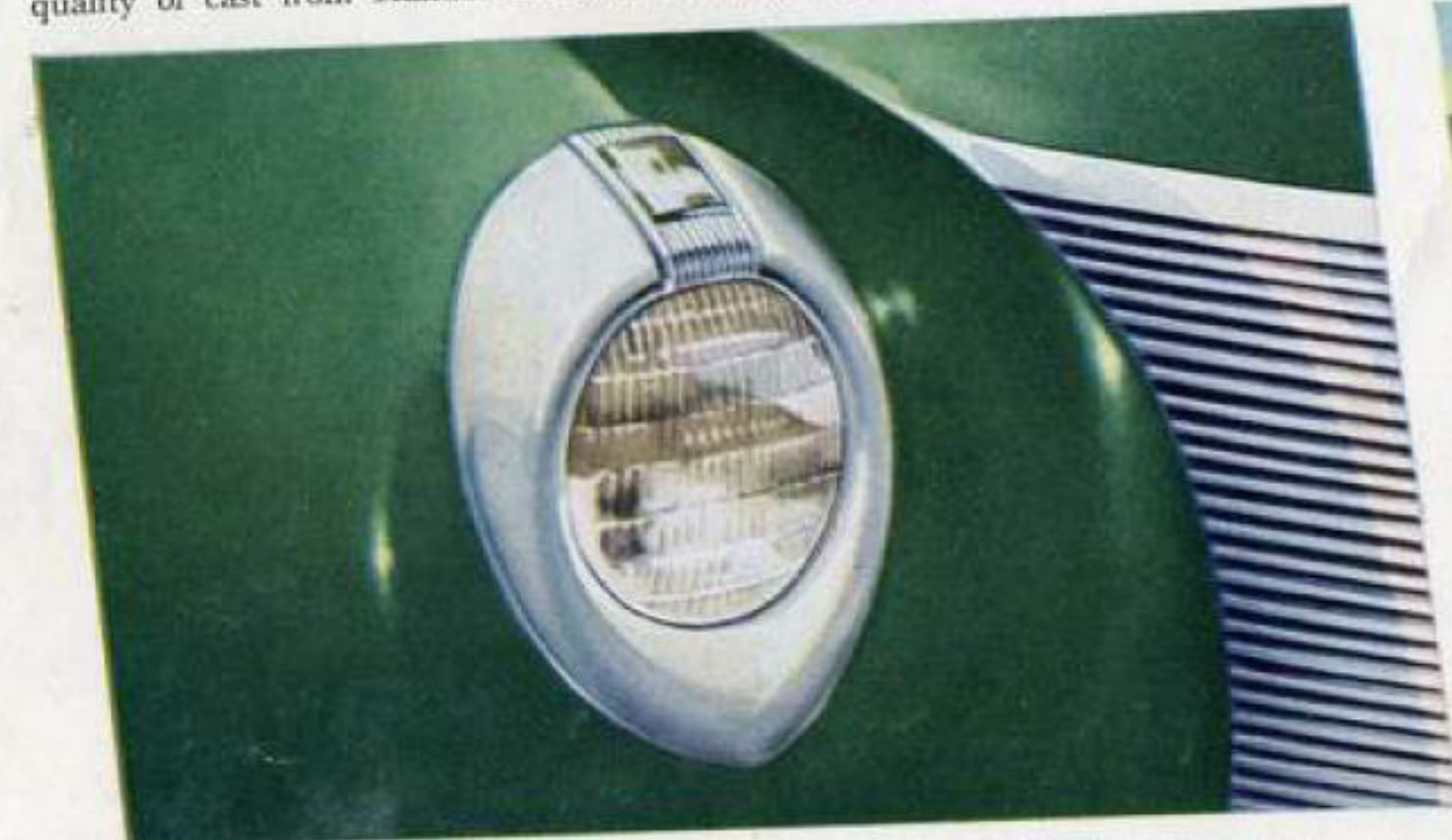
NEW SEALED-BEAM HEADLAMPS give 50% more light. Night driving safer because driver can see nearly twice as far ahead. Sealed construction insures longer life, prevents loss of lighting efficiency. Parking lamp with separate lens above headlamp.
