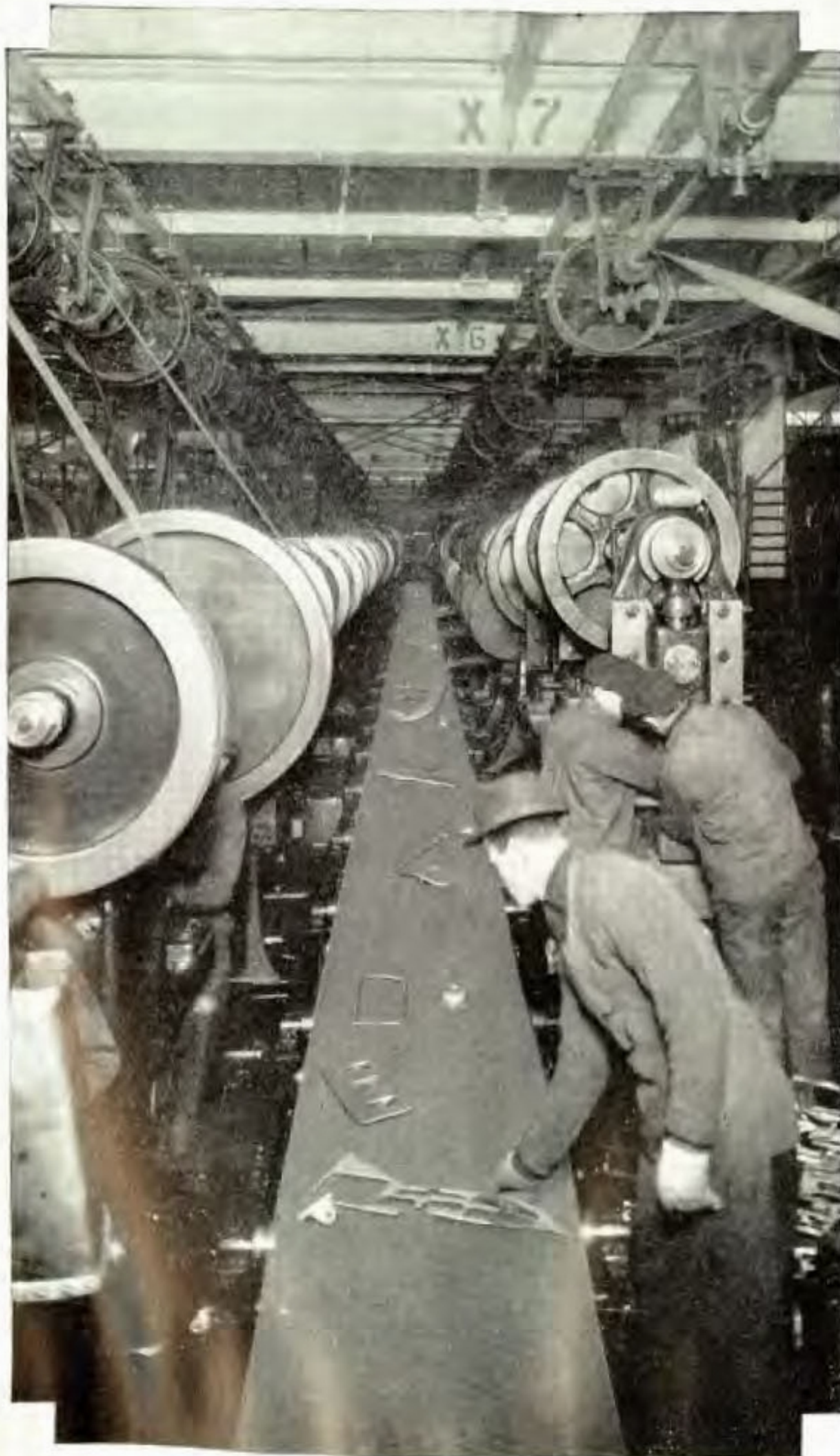
This Belt Carries the Finished Steel Parts and Scrap from the Punch Presses
