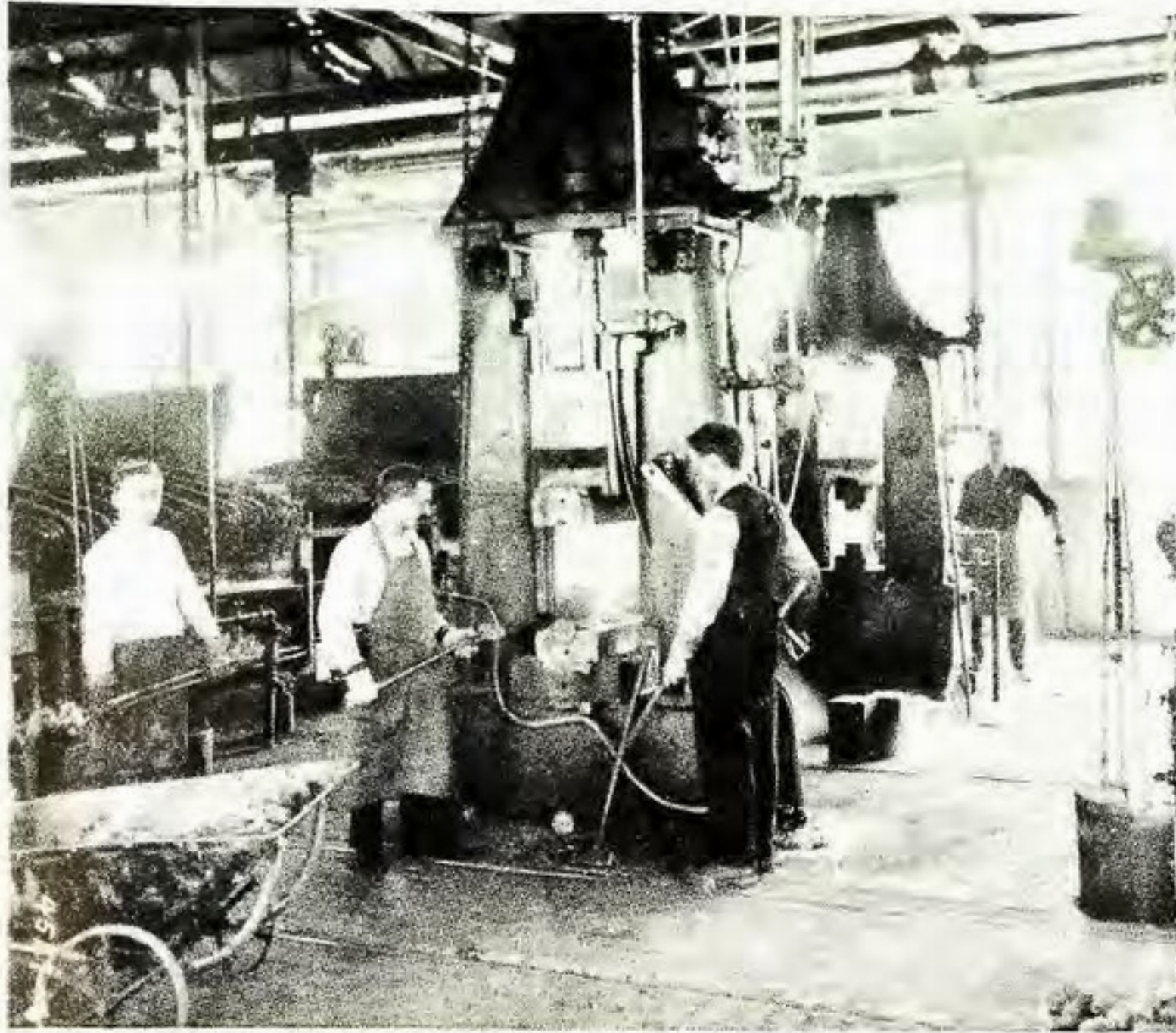
Restriking or Straightening Crank Shafts on Steam Hammers
