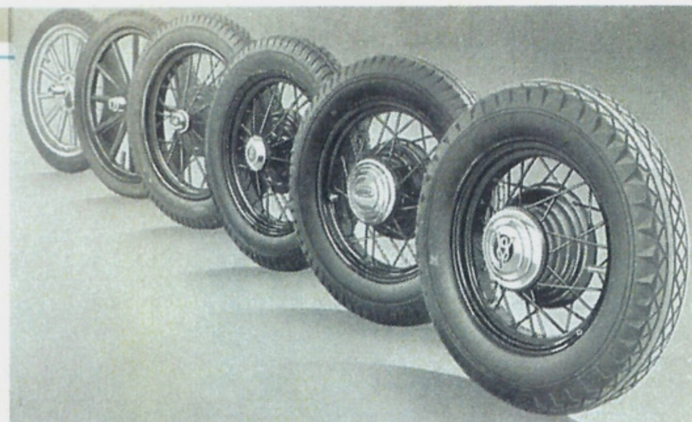
Thirty years of progress between the 28-inch wooden wheel with 3-inch tire of the 1903 Model A to the steel spoke one-piece electrically welded wheel of the 1933 Ford car with 5.50 x 17 balloon tires.
