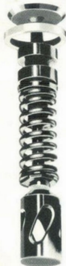
V-8 valve seat inserts are so hard that they will give 40,000 to 50,000 miles without attention. V-8 valves are "set" at the factory and in most cases will need no adjustment before 40,000 or 50,000 miles. This is a big improvement over ordinary valves which so soon become worn that they require adjustment to prevent loss of motor power and fuel wastage.
