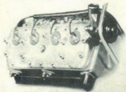
The dual down-draft carburetor and aluminum duplex intake manifold combine to feed the eight cylinders uniformly under all conditions. Through the use of a double carbureting and manifolding system NO two cylinders draw in succession from the same side of the carburetor or manifold. Atop the carburetor is an air intake silencer and cleaner.
