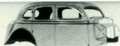
ONE PIECE, WELDED ALL STEEL BODIES.
