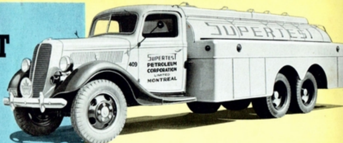
Supertest Petroleum Corporation, Limited of Montreal, haul a 1010-Imperial-gallon gasoline tank, as shown, with a 157-inch truck that has a two-speed axle and trailing third axle. The unit also has provision for carrying 1750 pounds of oil and grease.
