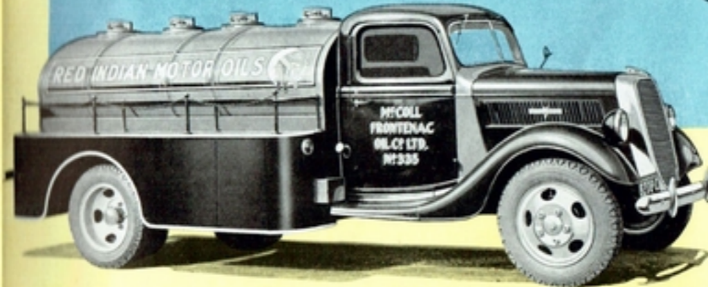
This Ford V-8 equipment is used by McColl Frontenac Oil Co., Ltd. This 157-inch De Luxe truck equipped with two-speed axle, hauls a 736-Imperial-gallon gasoline tank equipped with side racks to carry oil.
