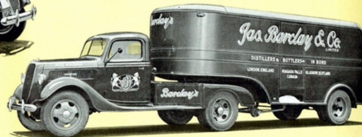
Operated by Jas. Barclay & Co., Limited, this Ford V-8 truck with drop frame semi-trailer van body combines utility with strong advertising display. Body measures 18' x 72' x 60'.
