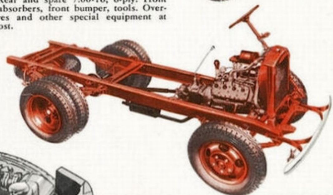
101 INCH C.O.E. CHASSIS (85 or 95 hp) Standard equipment: Cab, hood, front fenders; running boards; instrument panel; horn; lamps. 23 gallon fuel tank; spare wheel carrier; five wheels. Tires: Front 6.00-20, 6-ply. Rear 6.50-20 (32 x 6) 8-ply. Front bumper; jack and tool kit. Dual wheels, heavy-duty tires, spare tire, auxiliary springs, two-speed axle, frame reinforcements and other special equipment available at additional cost.
