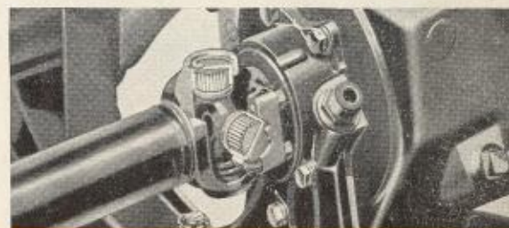
SMOOTH, EFFICIENT driving power is transmitted by tubular shafts, needle bearing universal joints and rubber encased centre bearing. Front joint is split type for easy servicing of clutch and transmission.
