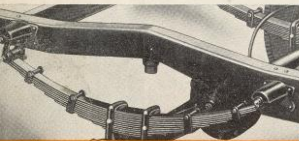
TRUCK-BUILT SPRING LEAVES are of special alloy steel with tensile strength of 200,000 lbs. per sq. in. Heavy spring brackets are securely attached to frame. Shackle pins have large bearing surfaces, and resist side thrust for greater riding stability.
