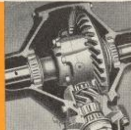
HEAVY 3/4 FLOATING TYPE REAR AXLE with straddle-mounted pinion. Differential carrier mounted on large tapered roller bearings, spaced to distribute load equally.
