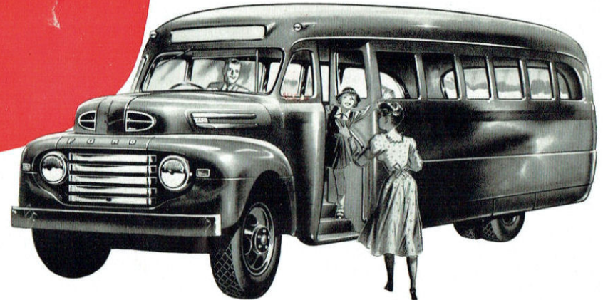
BUS CHASSIS, 14,500 lbs. G.V.W.—173" & 194" w.b.—Up To 27-Passenger
