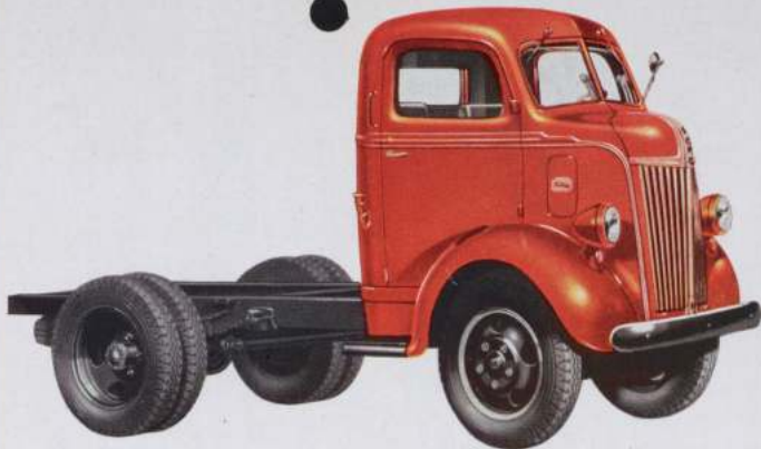
Ford 1½- and 2-ton cab-over-engine units for either truck or tractor service. Available with 100 H.P. V-8 engine, in 101", 134", and 158" wheelbases, with cab.
