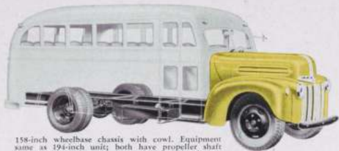
158-inch wheelbase chassis with cowl. Equipment same as 194-inch unit, both have propeller shaft and parking brake guards* and extended tailflap.
