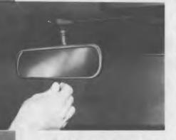
There's no need to suffer the annoyance of reflected glare from headlights behind you. You can virtually eliminate it simply by pressing on the tab at the base of this convenient mirror. Made with high grade, non-glare glass, it is excellent for daytime driving, too. Part Nos. BA-18400-C, BA-18400-D.
