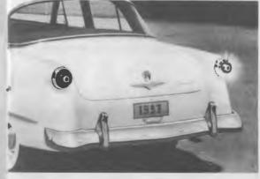
Signal your turns safely and conveniently-night and day-in any weather. A finger touch on the steering column control starts flashing light sig-nals in both front and rear of car. Cancels automatically when turn is completed. Part No. FAD-18440-A.
