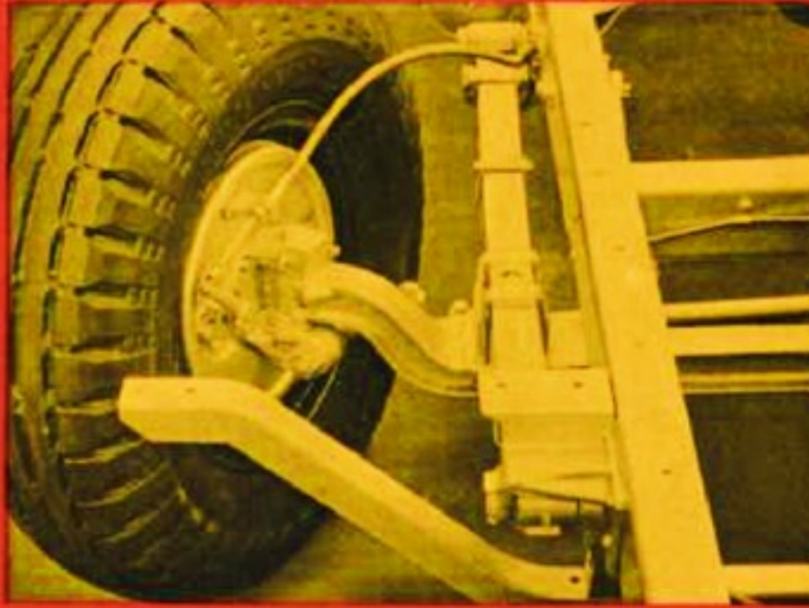
The heavy front axle is designed especially for equal load distribution on front and rear axles. Front brakes are controlled by cables and conduits.
