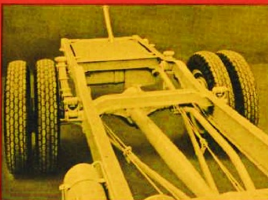
The rugged frame construction, full torque-tube rear axle and springs are illustrated here. Notice also the large size and protected mounting of the fuel tank.
