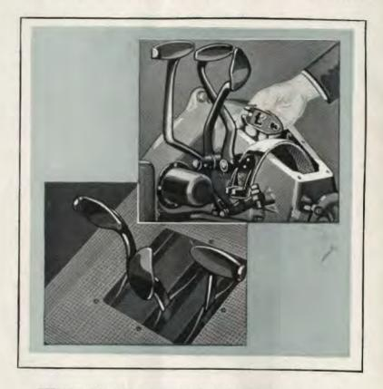
THE width of the transmission brake band has been increased to 13/4 inches, a feature which contributes to ease and smoothness of braking. All bands have removable ears to permit changing of lining in a few minutes, should occasion require it.
