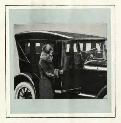
TOURING Car has four doors, making it easy for passengers to enter and leave. Close-fitting curtains open with the four doors and make the car practical and comfortable in cold or stormy weather. The light, strong top may be quickly lowered or raised for summer touring or sport usage.
