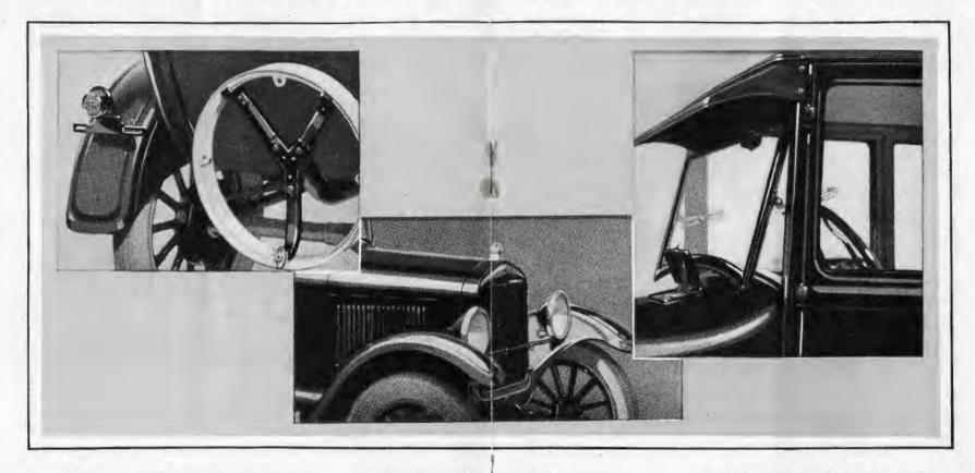
LARGE, powerful brakes of positive action make driving safe. The strong, simplified tire carrier accommodates either Ford wire wheel or demountable rim. Combination license bracket and tail light located on rear left fender. Note the large, wide fender construction.
