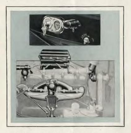
THE instrument board is arranged to provide the utmost convenience with ammeter and switches grouped in one panel. The choke button also controls the carburetor adjustment.
