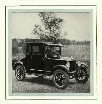
THE Coupe is an exceptionally good looking car for personal use. Finished attractively in color with upholstery to harmonize. The body, with graceful coupe pillars and excellent molding treatment, is of rigid all-steel construction. The large windows and one-piece windshield of fine plate-glass aid visibility.
