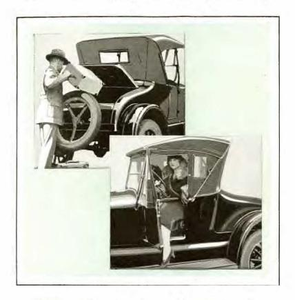
THE rear deck compartment of the Runabout has a capacity of 13 cubic feet, and will carry packages 16 inches high. The compartment is 42 inches wide and 44 inches long. Close-fitting curtains that open with the doors make driving comfortable and convenient in all kinds of weather.
