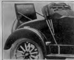
(Seat Open and Top in Place) Premier wire, woven in helical coil springs, used throughout in cushion and back. Trimmed with highly durable pebble grain leather cloth.
