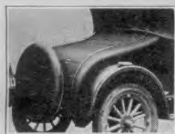
(Seat Folded Snugly into Place) Note the neat aluminum castings bolted to rear fender for step plates. Top support irons are also furnished.
