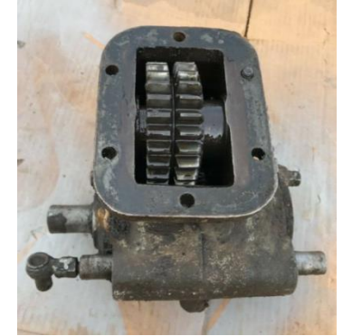
PTO to Drive Rear Equipment, mounted to right side of Transmission.
