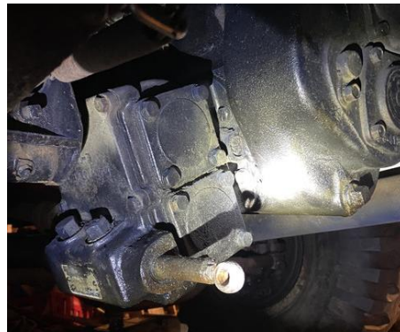
Braden/Arrow Gear PTO Model BHD 7 mounted to an NP420 on a WM300.
