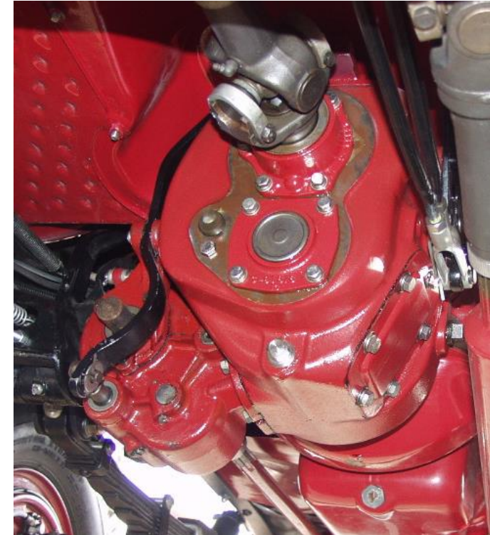
Detroit Harvester PTO Model 12546 used on the FFPW NP420 Transmission.
