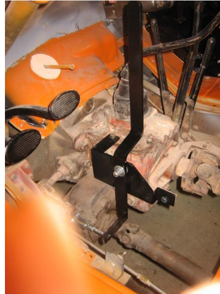
Fabricated bracket/lever to replace cable-controlled PTO.
