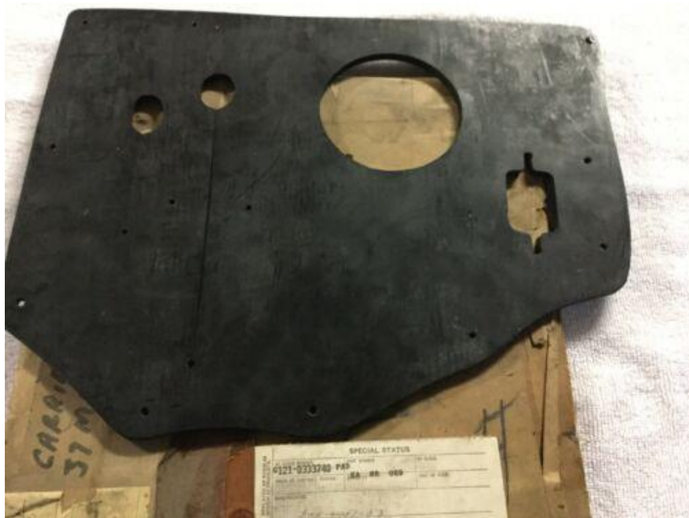
Transmission draft pad used on G121 - WW2 Dodge WC ¾ Ton Series (W55 [T214], Fargo Dodge) vehicles w/winch and WC-64, and KD Ambulance w/o winch and WC-54 Ambulance after S/N 81625758.
