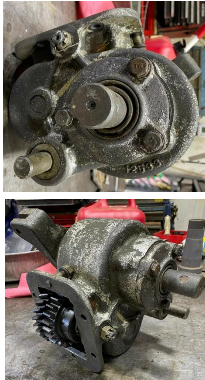
Detroit Harvester PTO Model 12533 used on the M37 NP420 Transmission.
