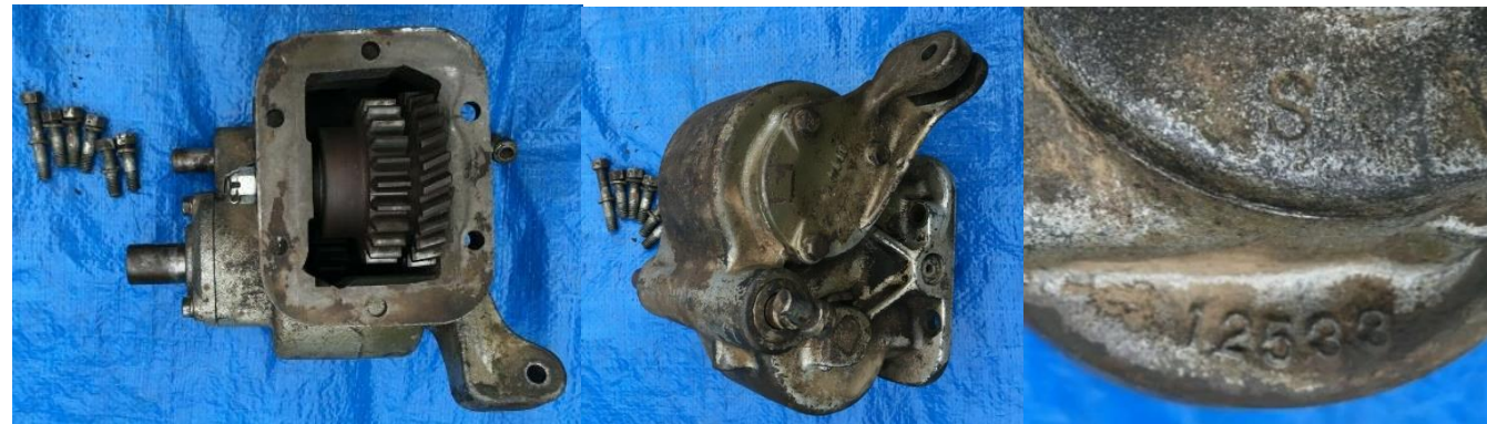
Detroit Harvester PTO Model 12533 used on the M37 88950 Transmission.
