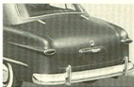
Streamlined rear deck hinges and handle blend neatly into deck lid.
