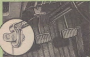
Hand brake cable reverses direction by running back over a free-turning pulley for easier operation, longer life.
