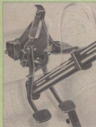
Foot pedals are suspended, avoiding holes in toe board, increasing driver's foot room, reducing effort required to operate.
