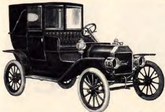
Model T Landaulet or Taximeter Cab 4 Cylinder 20 Horse Power $950.00 f. o. b. Detroit
