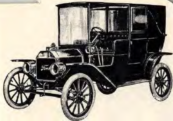
Model T Town Car 4 Cylinder 20 Horse Power 5 Passenger $1,000.00 f. o. b. Detroit
