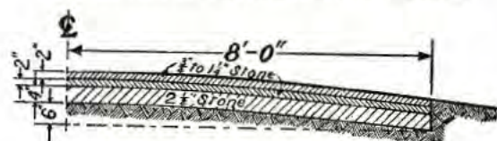
TYPICAL HALF SECTION BITUMINIZED MACADAM.
