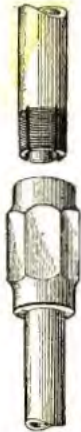
Fig. 4. Lock nut permitting adjustment of front stay rods to fit any car.
