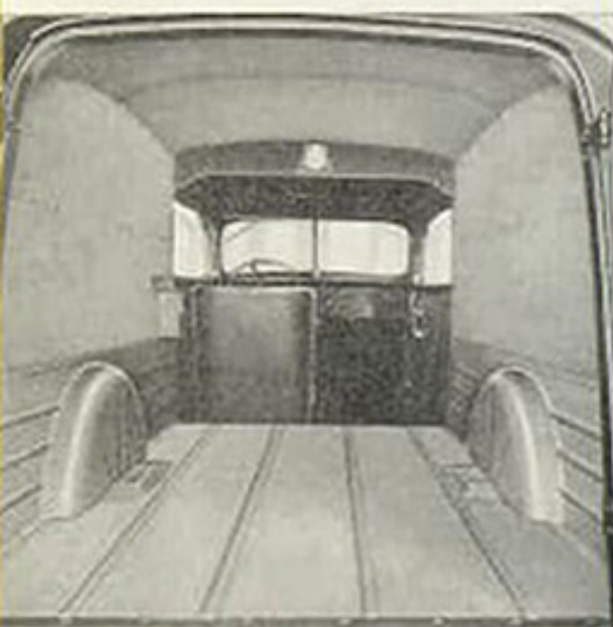
The Panel is available with durable, waterproof fibre board lining at low additional cost. The hardwood floor is protected by steel skid strips.
