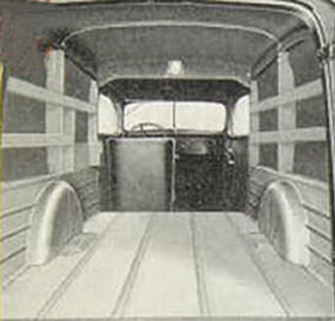
Panel body sides protected by steel lower panels and hardwood slats. Passenger seat at additional cost.
