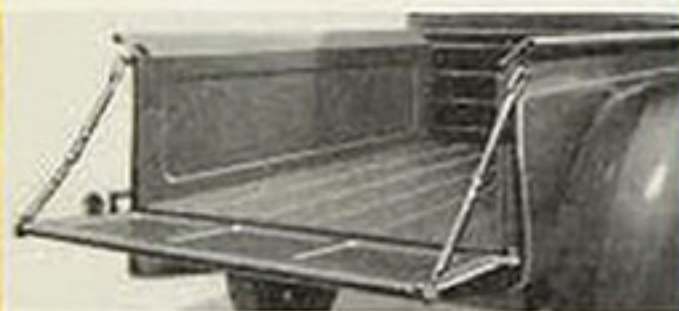
Pickup has sockets in flareboards for adding side boards, rack or top. Front panel, which is same height as flareboards, is strongly reinforced.
