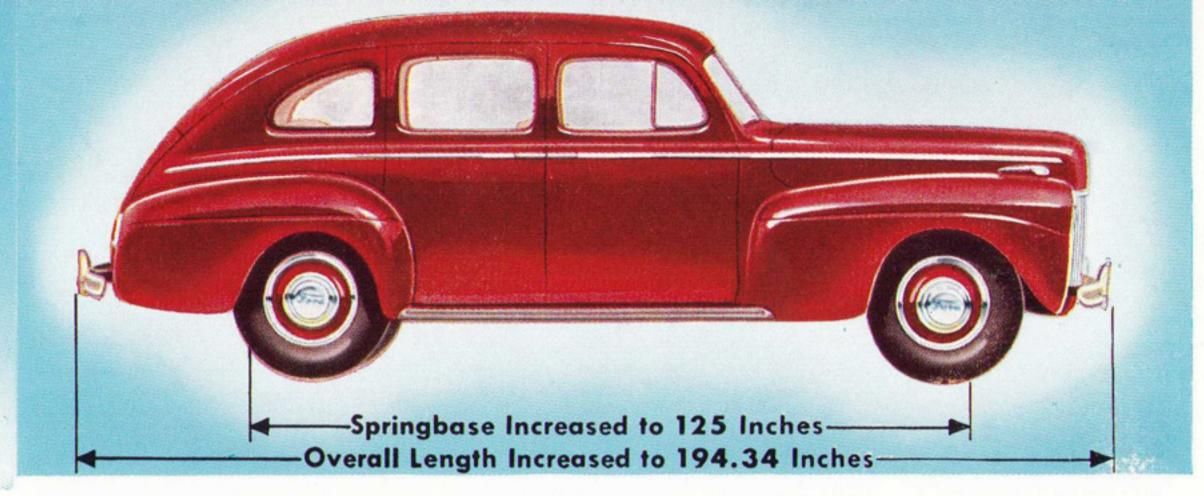
The increased length of the 1941 Ford contributes to its remarkable riding comfort. Springbase has been lengthened in proportion to the new longer wheelbase. Passengers are carried well ahead of the rear axle and spring, near the center of the car where the riding is best. And beneath the flowing beauty of this big car is a rigid new frame, twice as resistant to twisting force as the former rugged Ford frame.
