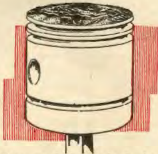
From actual photograph, showing carbon formation on head of piston
