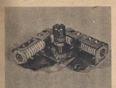
The Lincoln-Zephyr coil was manufactured for the use of resistance units, which in this case are two Ford coil resistors joined together as shown in photo to make up unit, which lets both coils get an equal amount of voltage. The main distributor lead is fastened to the center lug, which joins the resistors. Unit is fastened to coil by using two 8/32 nuts.
