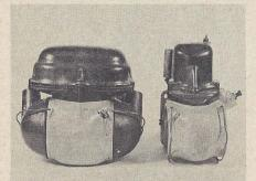
Shown here are the two stock distributors necessary for the conversion. The Lincoln distributor should, if possible, be procured complete with the coil, inner terminal plates, outer caps and a flawless distributor case. The Ford distributor may be either an 11-A (1937 to 1941 Ford) or a 40-B (1932 to 1936 Ford). Only the inner components will be used from either of these. The outer condition may be disregarded. Price on this item is from one to two dollars.
