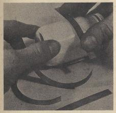
Pick-up prongs, which are brass, are given new surface by grinding wheel. This is done to all six prongs, at the same time retaining original angle or contour for rotor prongs. Remove only enough to give new surface on ends. Wire-brush the complete outer surface of pick-up prongs. This makes for better
