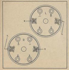
Locator notches (1, 1) are on the opposite side of plate. These must be located as shown here to differentiate right and left plates. Center terminals (2, 2) are blocked off with tape. Be sure to mark plates "Right" and "Left."
