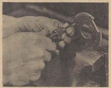
With drilling and tapping operation completed, check by holding a steelrule or similar straight-edge across the face of the plate to see if the plate is warped or uneven. File flush if uneven and polish if so desired. Install the plate in proper place in the distributor base. If a loose fit is encountered, gently peen edges of plate until a snug fit is encountered. This enables the points to retain their original settings.
