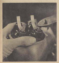
Excess metal at ends can now be trimmed off about ¼-inch from where outer prongs join strips.
