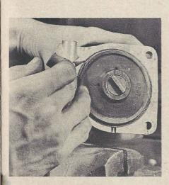
By checking to see if base is flush with case, where case mounts to timing gear cover, amount to be removed from distributor shaft where rotor mounts can be determined.
