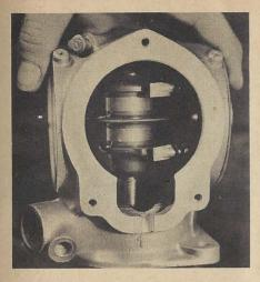
With rotor in place on distributor shaft, and shaft in base, install unit in Zephyr case. Inserting one of the newly converted terminal plates in its proper place, check rotor prong clearance, on new pick-up strips. If rotor prongs touch strips, band file enough of prong to just clear the strip. Prongs should come as close to contact with strips as possible without touching.
