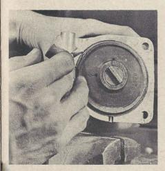
By checking to see if base is flush with case, where case mounts to timing gear cover, amount to be removed from distributor shaft where rotor mounts can be determined.
