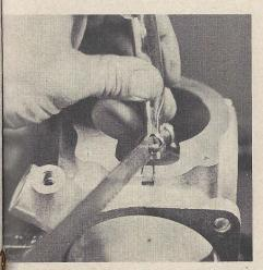
Quarter-inch wide by quarter-inch deep notch is hacksawed into case where back part of coil mounts. Slot is for new wires from condensers to points.
