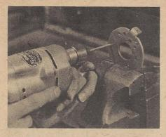
An 8-32 tap is used for installing new threads in newly drilled holes. When tapping is finished, chamfer tapped holes with a ¼" drill. By using this large a drill, the rough edges of newly tapped holes can be readily removed without cutting into threads. Easy does it at this point—a touch of the drill will do the job.
