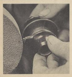
If rotor has not been previously ground, due to earlier rebuilding, grind ½2-inch from ends of prongs. Rotor should also be checked for cracks and carbon streaks.
