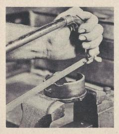
Ford base where ear of points-plate fits is lengthened by removing 1/8" with hacksaw, to allow a greater advance and retard range.
