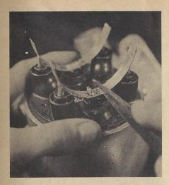
With strips now fastened on all prongs, remove excess solder from strips with bearing scraper, or sharpened threecorner file.
