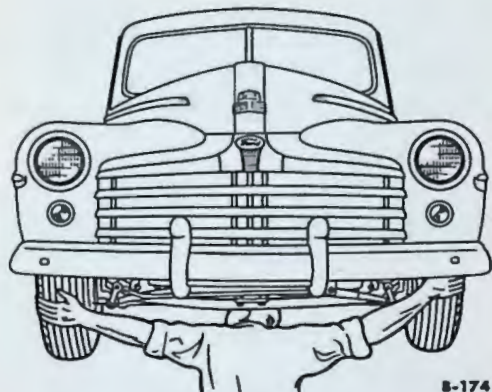
Fig. 4—Checking Tie Rod and Drag Link Ends
