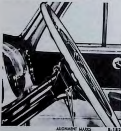
Fig. 2—Steering Wheel Alignment Marks
