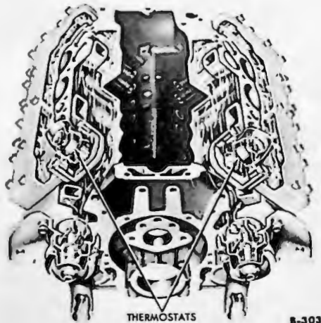
Fig. 5—Series Flow Cooling
